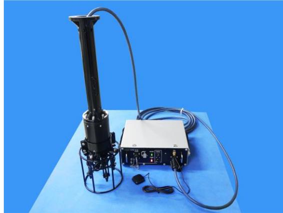
This system can detect the presence of dolphins, find out the direction and track dolphins by receiving their sound waves. 4 hydrophones array are designed to determine the arrival direction of dolphin's sound using correlation processing.
